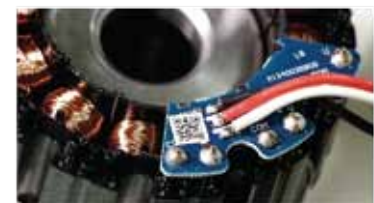
Data management with our QR Code system in each process step to ensure quality and traceability for every single product.
