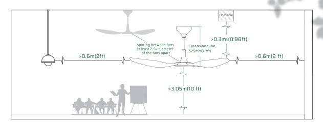
$<sup>\</sup>ensuremath{\mathtt{\#}}$  The above specifications are test from SUNON Lab and the data will be affected by different environmental conditions.
