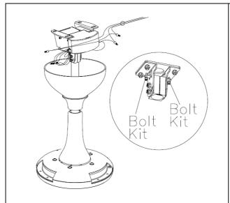
9-1 Loosen attach bolt kits on yoke, raise the canopy, then secure it to the fixed bracket.
